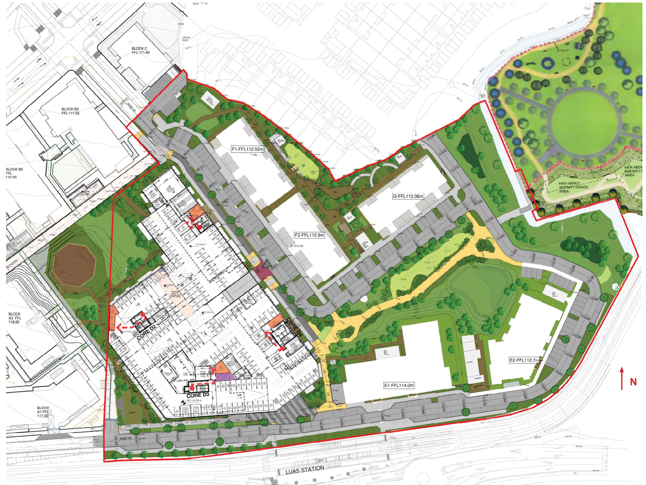
Figure 30 - Basement Floor Plan with waste storage areas highlighted
